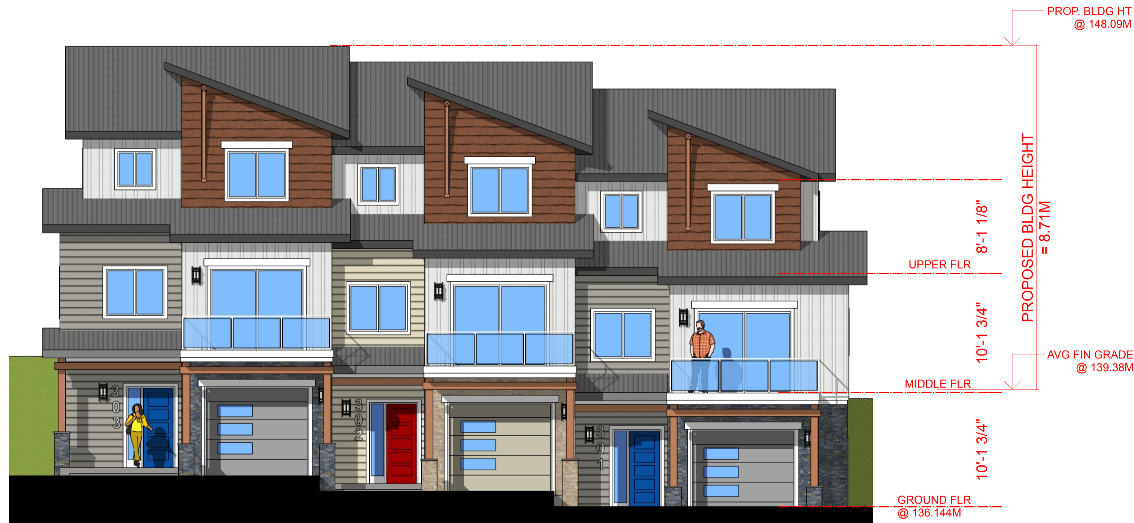
FRONT ELEVATION (NORTH) 3/16" = 1'-0"
